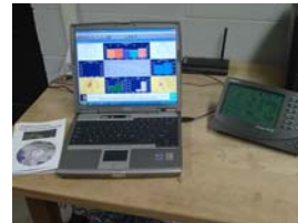
Figure 2. Davis Vantage Pro2 console and laptop with analysis software.
